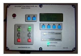
Front Panel Switches, Input And Output Monitors
