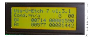
Line 1 – Current firmware revision Line 2 – Conductivity value and regeneration status Line 3 – Oxidizer valve status, current/last flow counts, flow counts since power on or reset. Line 4 – Acid valve status, current flow counts, flow counts since power on or reset.
