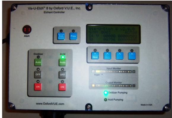
**Front Panel Switches, Input And Output Monitors**
